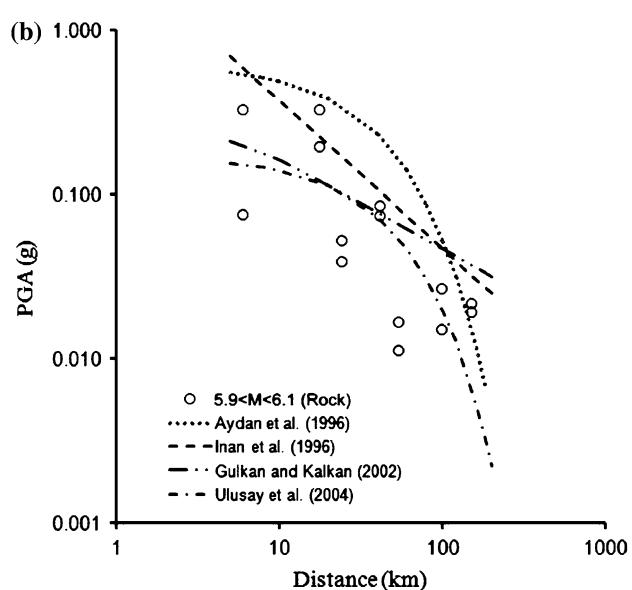
**Fig. 13** Comparison between predicted PGA values by domestic attenuation relationships and PGA values of true earthquake records for rock sites: **a**  $M_w: 5.0 \pm 0.1$  earthquakes; **b**  $M_w: 6.0 \pm 0.2$  earthquakes
