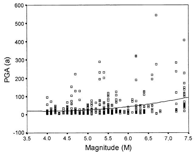
**Fig. 9** Peak horizontal ground acceleration versus magnitudes for data from Turkey (magnitudes as recorded)
