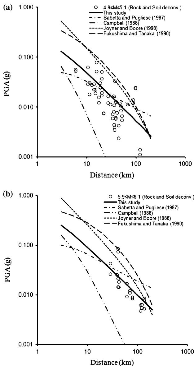
**Fig. 19** Comparison between imported relationships and rock site data plus transformed soil site data, including the results from this study: **a**  $M_w: 5.0 \pm 0.1$  earthquakes; **b**  $M_w: 6.0 \pm 0.1$  earthquakes
