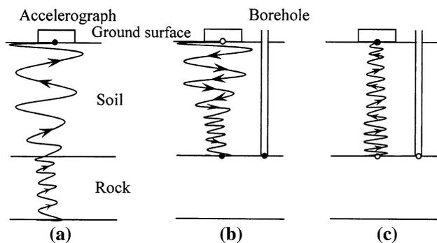
**Fig. 7** Schematic illustration of data transformation through Pro-Shake. **a** Accelerograph record at top of a soil column; **b** transformation of seismic record to desired level; **c** carrying back the transformed record to the ground surface as it was recorded on a rock site
