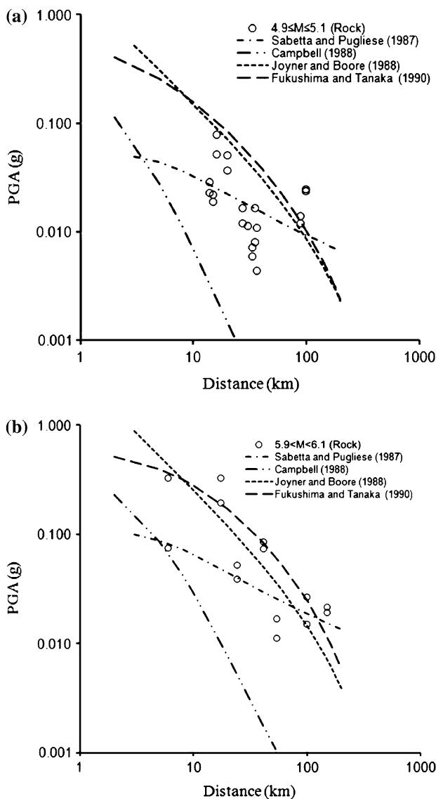
**Fig. 15** Comparison between PGA values predicted by imported relationships and true records from Turkish rock sites: **a**  $M_w: 5.0 \pm 0.1$  earthquakes; **b**  $M_w: 6.0 \pm 0.2$  earthquakes
