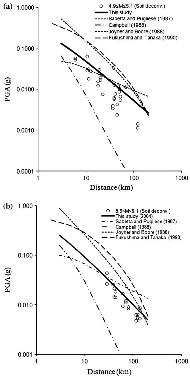
**Fig. 18** Comparison between imported relationships and soil site data (transformed), including the results from this study: **a**  $M_w: 5.0 \pm 0.1$  earthquakes; **b**  $M_w: 6.0 \pm 0.1$  earthquakes
