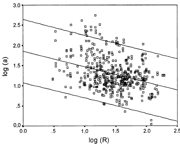
**Fig. 11** Log (PGA) vs. log ( $R$ ) for 95% confidence interval. The *middle curve* represents the average; the *upper* and *lower* ones stand for threshold values
