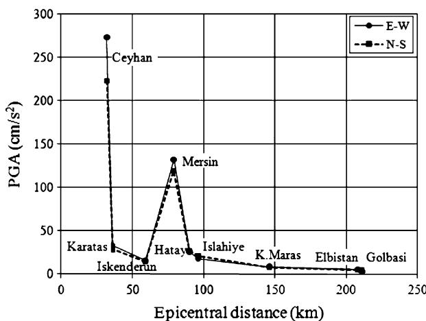
**Fig. 2** Site amplification effects for the June 27, 1998 Ceyhan earthquake
