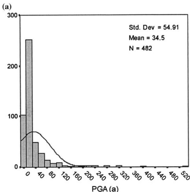
**Fig. 8** Histogram of peak horizontal ground accelerations from all sites in Turkey. **a** Inappropriate normal distribution; **b** log-normal distribution (units are  $\text{cm}/\text{s}^2$ )
