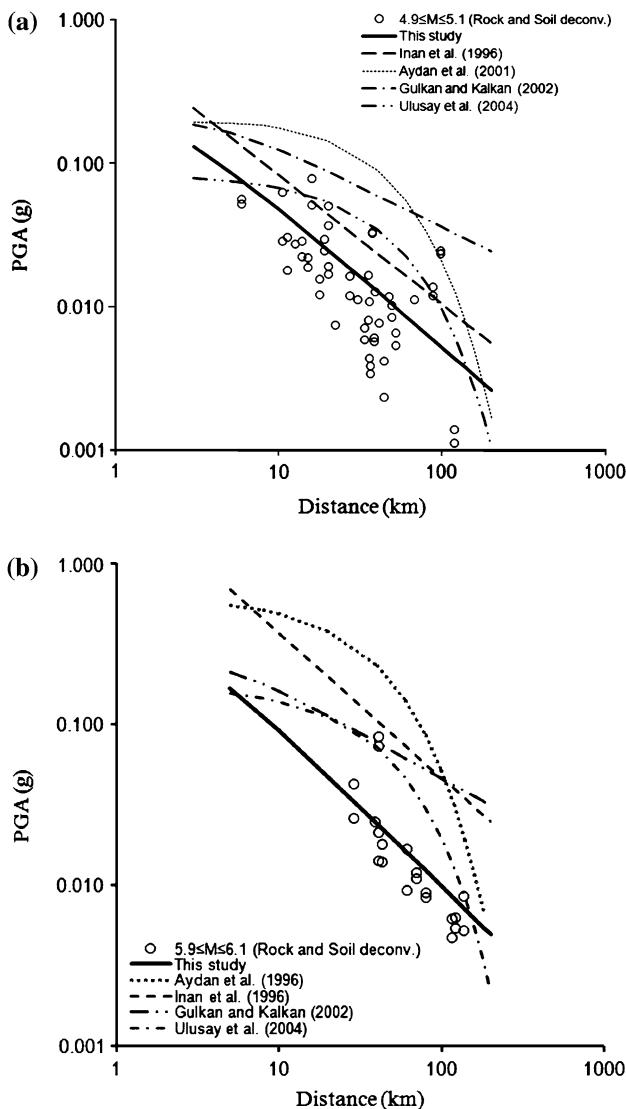
**Fig. 17** Comparison between domestic relationships and rock site data plus transformed soil site data including the results from this study: **a**  $M_w: 5.0 \pm 0.1$  earthquakes; **b**  $M_w: 6.0 \pm 0.1$  earthquakes
