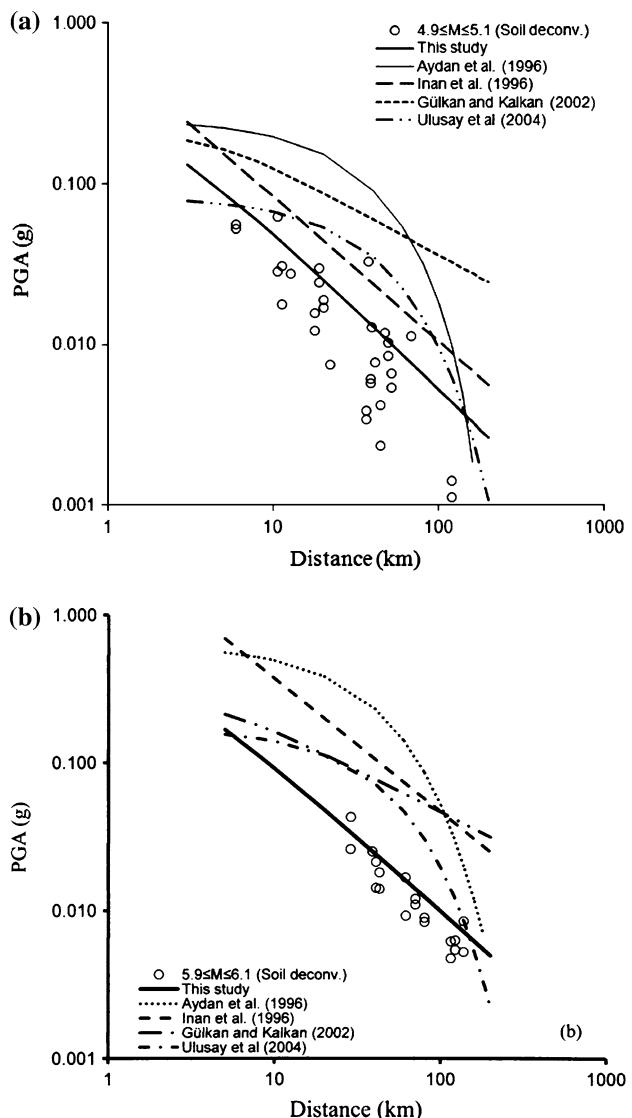
**Fig. 16** Comparison between domestic relationships and soil site data (transformed), including the results from this study: **a**  $M_w: 5.0 \pm 0.1$  earthquakes; **b**  $M_w: 6.0 \pm 0.2$  earthquakes
