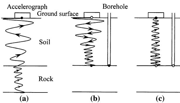
**Fig. 7** Schematic illustration of data transformation through Pro-Shake. **a** Accelerograph record at top of a soil column; **b** transformation of seismic record to desired level; **c** carrying back the transformed record to the ground surface as it was recorded on a rock site
