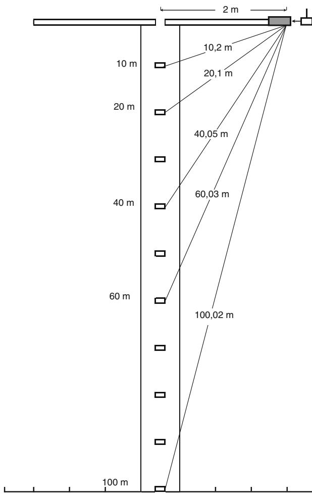
**Fig. 6** Schematic illustration of the down-hole technique used for field investigation
