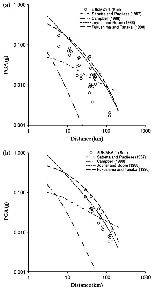
**Fig. 14** Comparison between PGA values predicted by imported relationships and true records from Turkish soil sites: **a**  $M_w: 5.0 \pm 0.1$  earthquakes; **b**  $M_w: 6.0 \pm 0.1$  earthquakes
