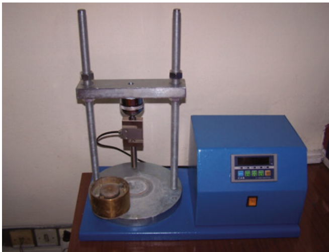
Fig. 1. Swell pressure measurement apparatus devised for this study.
