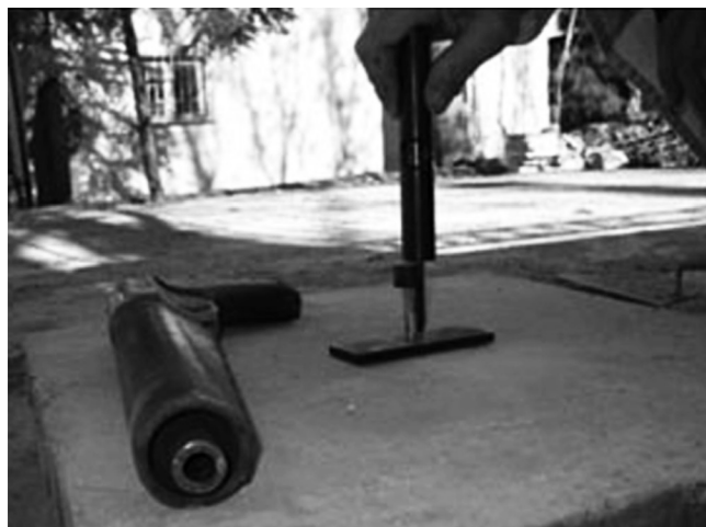
Fig. 2—Application of Windsor probe test.
